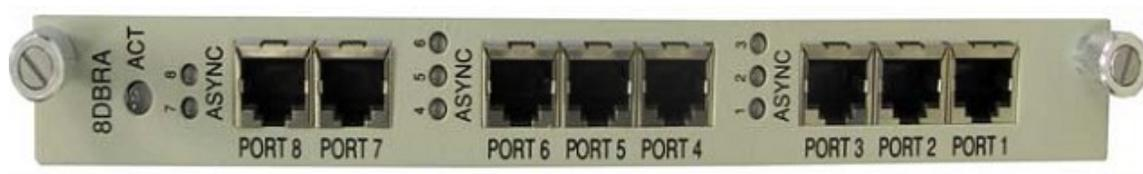
Since 1+1 Port Backup was selected, host ports 1 & 5, 2 & 6, 3 & 7, 4 & 8 are bridged. Host data transmitted into either port and is received downstream via the Virtual Port time slots mapped to the T1 DS-0s. Remote terminal responses are received on both of the paired ports.
