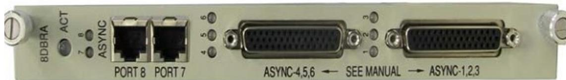
The 8DBRA card with the 8 RJ45 connectors provides easier, cleaner looking connections.
